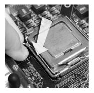
Press the four hooks down to fasten the cooler. Then rotate the locking switch (refer to the correct direction marked on it) to lock the hooks.  Align the holes on the mainboard with the heatsink. Push down the cooler until its four clips get wedged into the holes of the mainboard.
